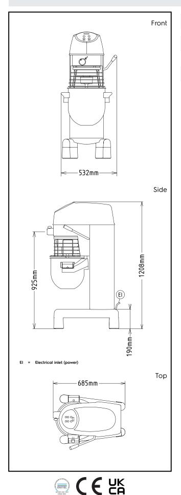
Electric Supply voltage: 200-240 V/1N ph/50/60 Hz Capacity: Performance (up to): 7 kg/Cycle 30 litres Capacity:
